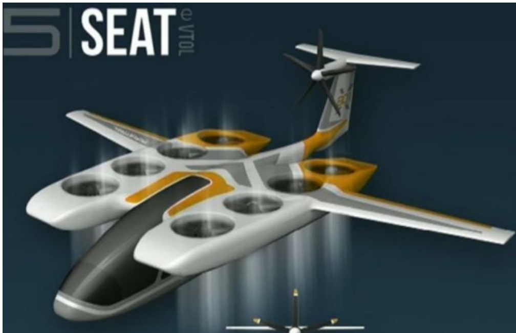
Figure 24 Distributive propullsion system.
