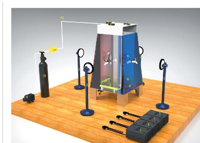
Figure 4 Experimental set-up of novel pyramid photobioreactor
