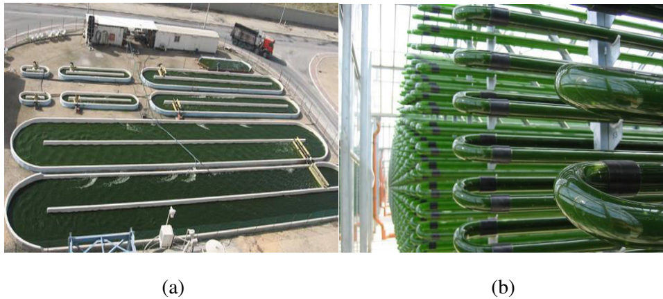
Fig.2 Examples of cultivation system: (a) open system (raceway ponds) and (b) closed system (tubular photobioreactor)
